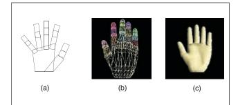
1. Hand models. (a) Cardboard model, (b) wireframe model, and (c) polygon-mesh model.
