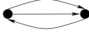
Fig. 7. Example that illustrates a FIFO-stable network, usually called \mathcal{U}_1 , which is not WC-stable. Specifically, there is an AQM adversary \mathcal{A} of rate r > 0.841 and a scheduling policy NTG-LIS (in NTG-LIS , the highest priority is assigned to the packet that still has to cross the smallest number of edges, solving ties by giving priority to the packet that has been in the system the longest time) such that (\mathcal{U}_1, \mathcal{A}, \text{NTG-LIS}) is unstable [54, Theorem 3].
