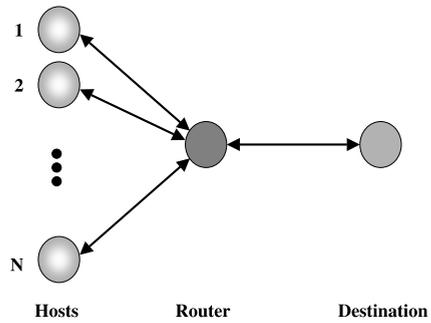
Fig. 2. The picture shows the interconnecting topology of the network we use in the proposed model.  $N$  hosts try to access a common communication link through a router. This router has a finite buffer which drops packets when it is full. All lines have the same capacity  $C$ .
