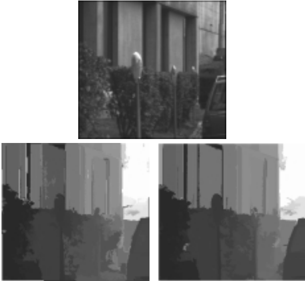
Fig. 5. Example “parking meter” from the JISCT test set [3]. Top: reference image; bottom left and right: depth maps obtained from the previous and new algorithms, respectively.
