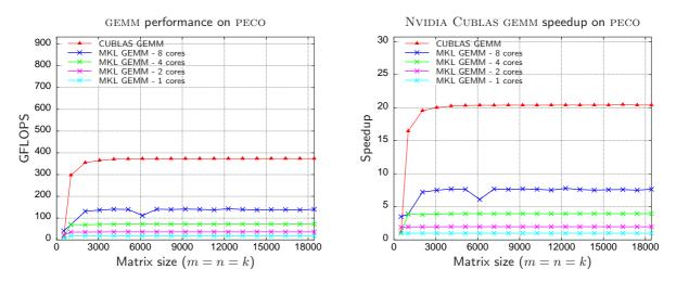
Figure 3.1: Performance of NVIDIA CUBLAS GEMM and Intel MKL implementation on 1, 2, 4 and 8 cores for square matrices (left). Speedups (right) consider the serial MKL implementation as a reference.
