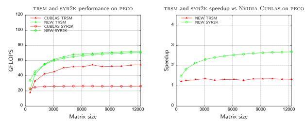
Figure 3.18: Performance of the tuned TRSM and SYR2K implementation on double precision matrices (left) and speedup compared with NVIDIA CUBLAS (right).
