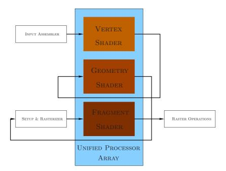
Figure 2.4: Cyclic approach of the graphics pipeline in the unified architectures.
