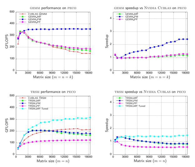
**Figure 3.16:** Top: Performance (left) and speedup (right) of the three variants for the GEMM implementation. Bottom: Performance (left) and speedup (right) of the three variants for the TRSM implementation.
