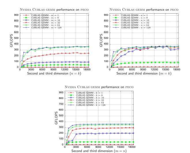
Figure 3.4: Performance of the GEMM implementation in NVIDIA CUBLAS for rectangular matrices. Top-left: m dimension is fixed. Top-right: n dimension is fixed. Bottom-center: k dimension is fixed.
