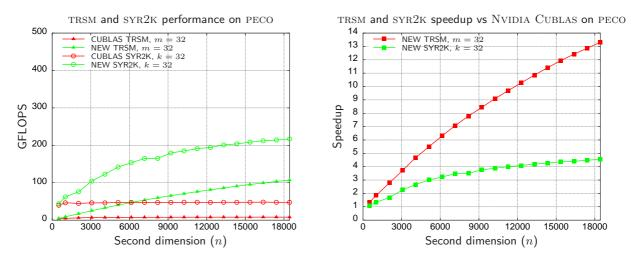
Figure 3.17: Performance of the tuned TRSM and SYR2K implementation on rectangular matrices (left) and speedup compared with NVIDIA CUBLAS (right).
