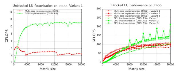
**Figure 4.10:** Performance of the single-precision unblocked (left) and blocked (right) LU factorization on the multi-core processor and the graphics processor on PECO.
