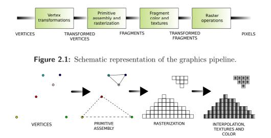
Figure 2.2: Operands of each stage of the graphics pipeline implemented by modern GPUs.
