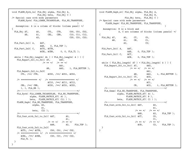
Figure 5.3: FLASH implementation of the function FLASH\_Syrk involved in the algorithm-byblocks for Variant 1 of the Cholesky factorization.
