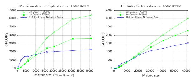
**Figure 6.15:** Performance of the device-centric implementation of GEMM (left) and the Cholesky factorization (right) compared with that of PLAPACK on 128 cores of LONGHORN.
