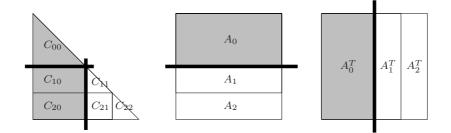
Figure 3.9: A visualization of the algorithm for matrix-panel variant of SYRK.
