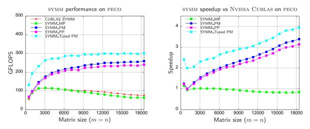
Figure 3.14: Performance (left) and speedup (right) of the three variants for the SYMM implementation.
