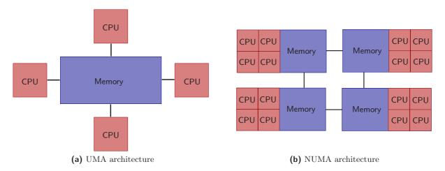
Figure 6.1: Shared-memory architectures. UMA (a) and NUMA (b) implementations
