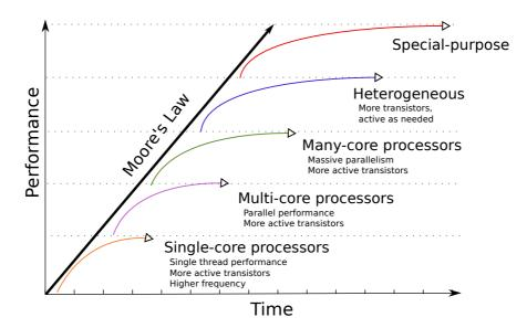
Figure 1.1: Evolution in performance of processor designs in response to Moore's Law. Figure based on a slide from P. Hofstee, IBM Austin.
