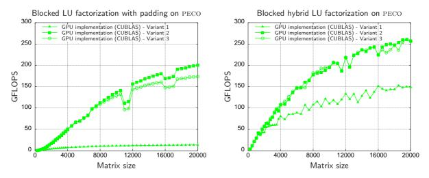
**Figure 4.12:** Performance of the single-precision blocked LU factorization with padding (left) and hybrid approach (right) on the graphics processor on PECO.
