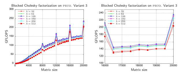
**Figure 4.5:** Impact of the block size on the single-precision Cholesky factorization using the graphics processor on PECO.
