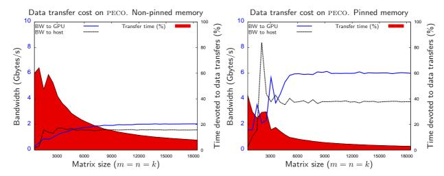
**Figure 3.6:** Percentage of time devoted to data transfers for the matrix-matrix multiplication. The plots include the effective bandwidth offered by the PCI-Express bus using *non-pinned* memory and *pinned* memory (left and right, respectively).
