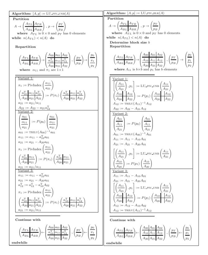
Figure 4.9: Algorithmic variants for the scalar (left) and blocked (right) algorithms for the LU factorization with partial pivoting.
