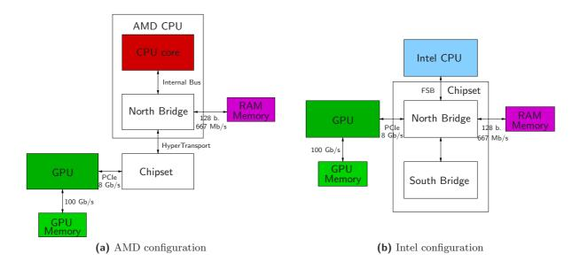
Figure 2.6: Examples of two contemporary architectures for hybrid CPU-GPU systems. (a) with an AMD CPU; (b) with an Intel CPU.
