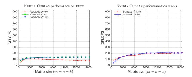
Figure 3.5: Performance of the Level-3 routines in NVIDIA CUBLAS for square matrices. Left: SYMM, SYRK and SYR2K. Right: TRMM and TRSM.
