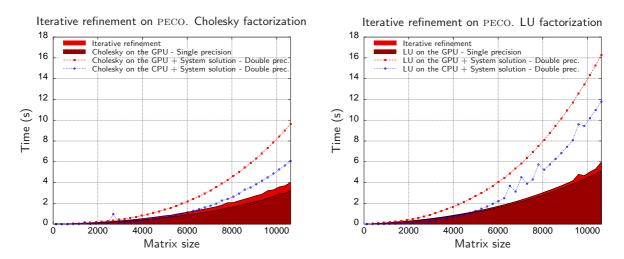
**Figure 4.13:** Time devoted to factorization and solution of a linear system using double precision on the CPU and the GPU, single precision on the GPU and an iterative refinement strategy on PECO. The Cholesky factorization (left) and the LU factorization (right) are employed to decompose the system matrix.
