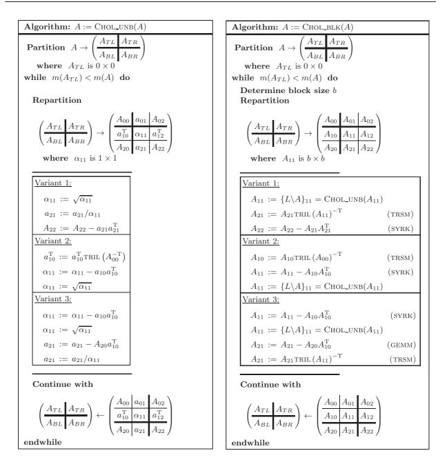
Figure 4.1: Algorithmic variants for the scalar (left) and blocked (right) algorithms for the Cholesky factorization.
