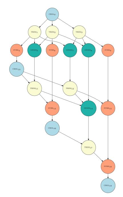
**Figure 5.4:** DAG for the Cholesky factorization of a  $4 \times 4$  blocked matrix.
