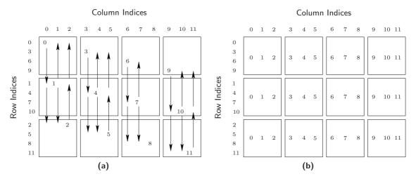
Figure 6.7: Spreading a vector within columns of processes.
