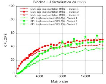
**Figure 4.11:** Performance of the double-precision blocked LU factorization on the multi-core and the graphics processor on PECO.
