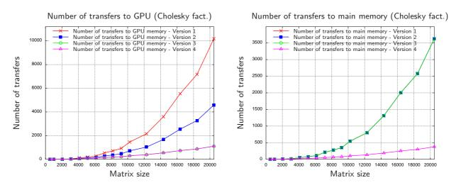
Figure 5.8: Number of data transfers for the Cholesky factorization using 4 GPUs on TESLA2. Block size is b = 768.
