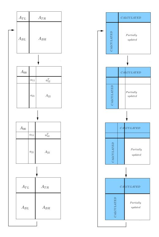
Figure 1.3: Matrix partitions applied to matrix A during the algorithm of Figure 1.2.
