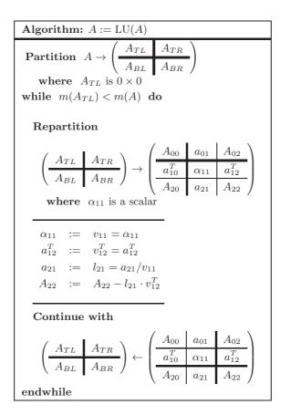
Figure 1.2: Algorithm for the LU factorizaction without pivoting using the FLAME notation.
