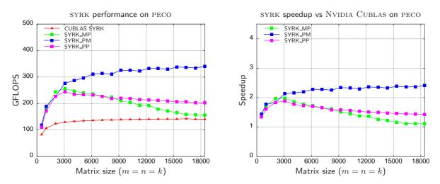
Figure 3.13: Performance (left) and speedup (right) of the three variants for the SYRK implementation.
