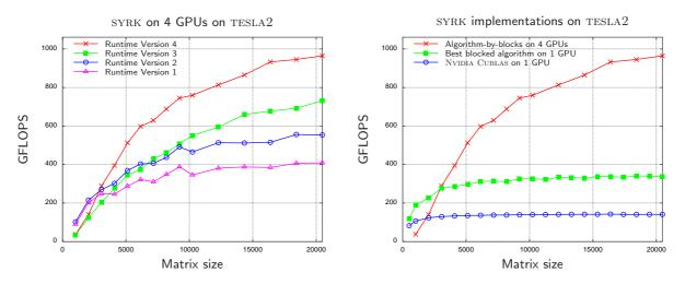
**Figure 5.16:** Performance (left) and comparison with mono-GPU implementations (right) of the SYRK implementation using 4 GPUs on TESLA2.
