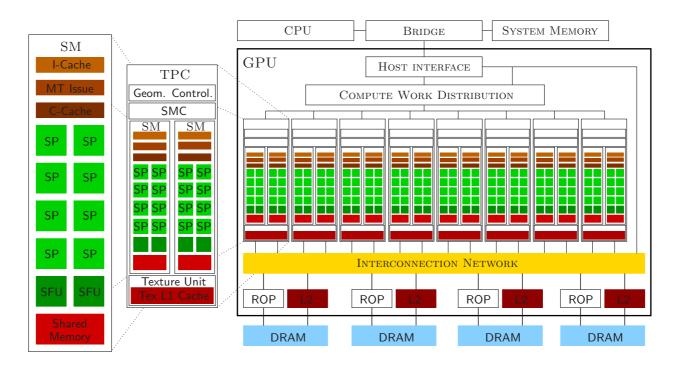
Figure 2.5: Unified architecture implementation on the NVIDIA TESLA series.
