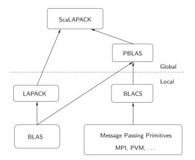
Figure 6.3: ScaLAPACK software hierarchy.
