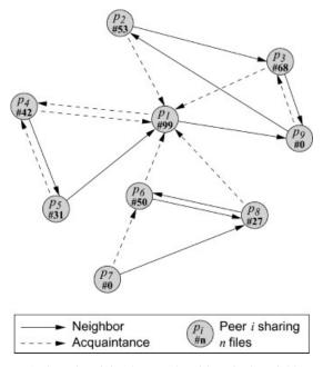
Figure 1. Sample minimal network, with a single neighbor and acquaintance link per peer.
