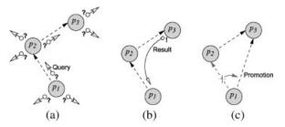
Figure 2. Basic principle of dynamic topology adaptation: (a)  $p_1$  issues a query. (b)  $p_3$  returns a positive response. (c)  $p_1$  promotes  $p_3$  as acquaintance.
